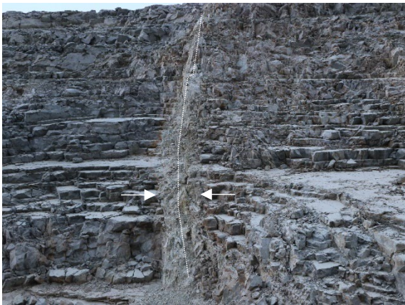
M. Favourable fault with RQD_{100} = 0 due to crushed rock (width 1 m) striking into slope in quartzite, Australia.
