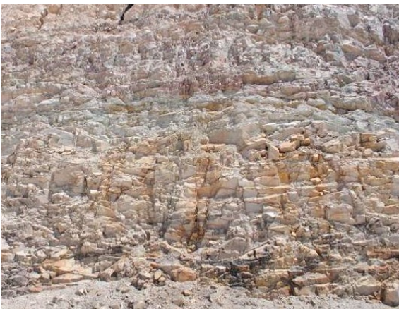
G. J_n = 12 . RQD: 75-90%. Three joint sets and random joints in sub-horizontally bedded sandstone, Australia
