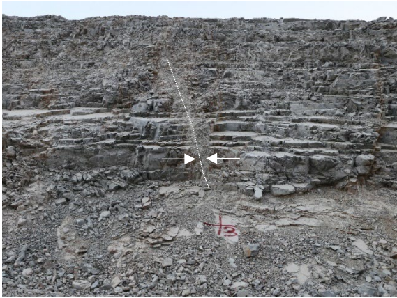
L. Favourable fault striking into slope with no clay (width <20 cm) in quartzite, Australia.
