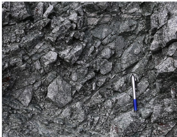
H. J_n = 15 . RQD=0%. Heavily jointed granodiorite adjacent to regional scale fault zone (note: pen for scale), Papua New Guinea.
