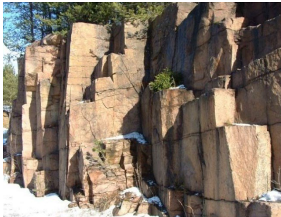
F. J_n = 9 . Three joint sets forming cubical blocks in granite, RQD=100%, Norway.
