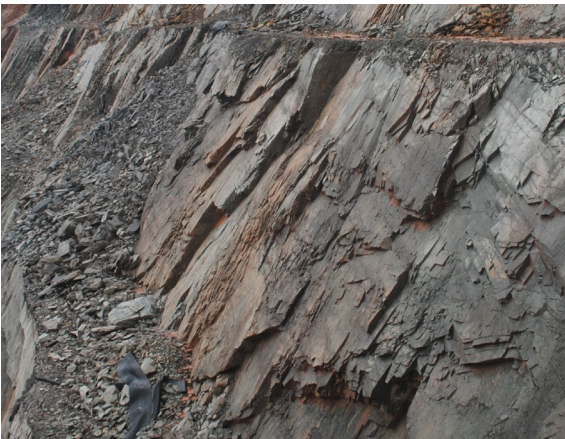
E. J_n = 6 . Two joint sets (foliation sub-parallel to slope and vertical joints striking into slope) and random joints in phyllite, Australia.
